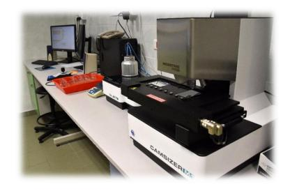
**Particle X-Plorer** software by **MICROTRAC** allows analysis of each tested particle by taking 50 different measurements from basic surface type and equivalent diameter to Feret length. Average measurement speed is from 16,000 to 1,000 particles per minute in a sample.
