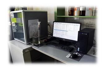
The apparatus handles a wide range of solid sample weights (up to approx. 2 g soil and approx. 400 mg organic material). Also measures the content of elements in liquid samples, provided concentrations are relatively high (i.e. within the lower measurement range).
