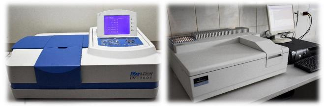
(UV/VIS). Capable of continuous measurement with scanning function, making them widely applicable for colorimetric analyses of water and water extracts.
