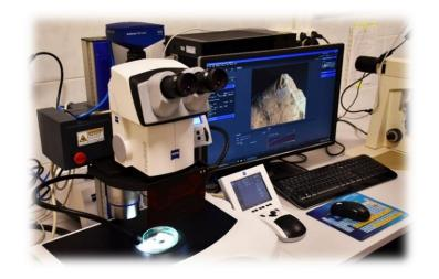
microscope and a workstation with **Zen Core** software allow high-quality documentary photos to be taken, experiments to be programmed and conducted, and analytical work to be conducted on collected material, such as size measurement, colour correction, etc.
