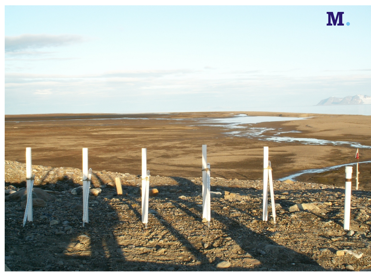
Photos 1-3 Ground thermometers on the Kaffiøyra: the beach site (B), the moraine site (M) and the tundra site (T).
