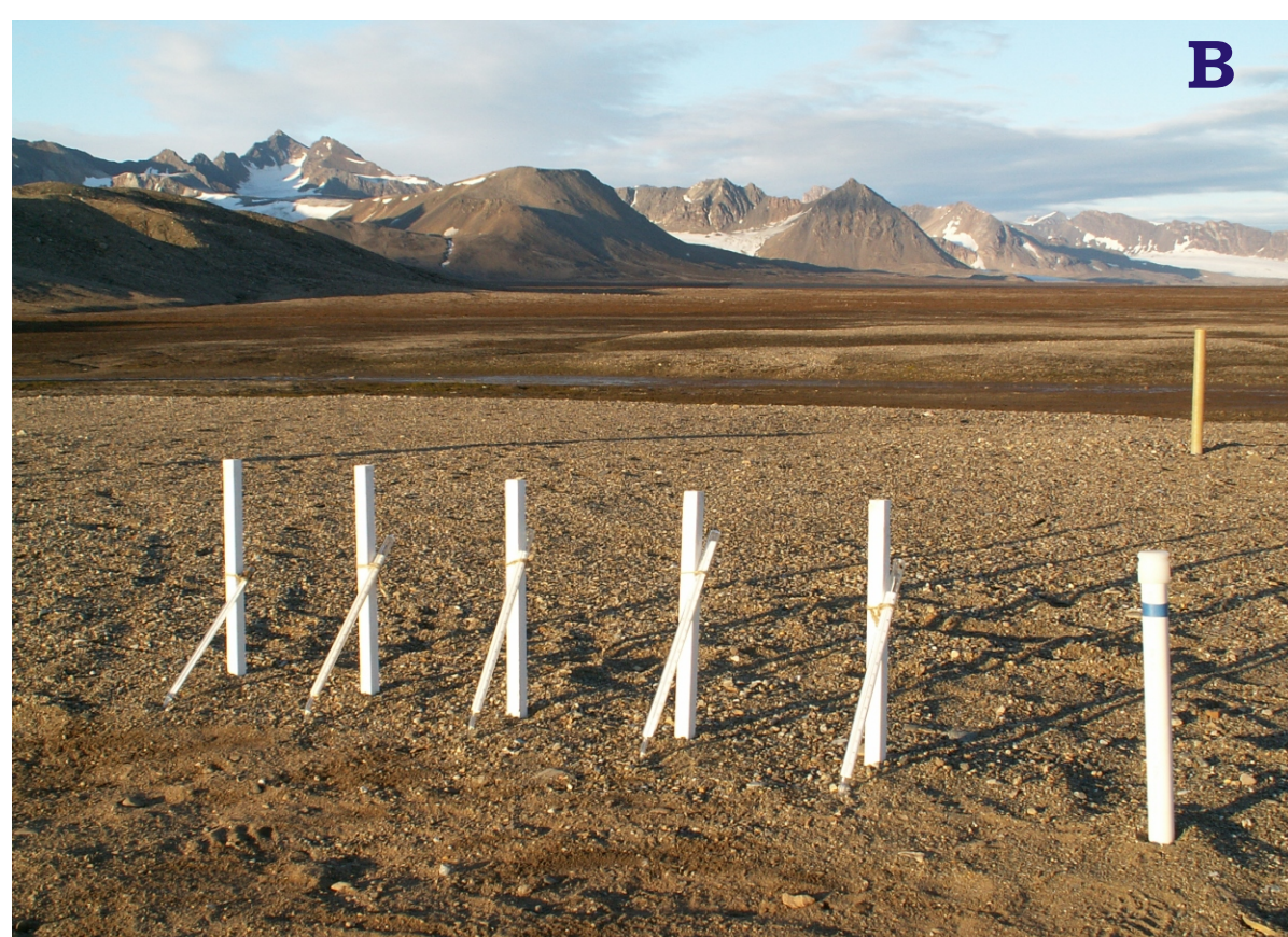
Photos 1-3 Ground thermometers on the Kaffiøyra: the beach site (B), the moraine site (M) and the tundra site (T).
